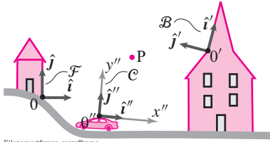
Figure 17.21: A third reference frame \mathcal{C} is defined by an origin O'' and coordinate axes x''y''z'' or base vectors \hat{i}''\hat{j}''\hat{k}'' . In this case \mathcal{C} is moving and rotating with respect to \mathcal{F} and \mathcal{B} . Once the x''y'' (or \hat{i}''\hat{j}'' ) directions are chosen the z'' (or \hat{k}'' ) direction is implicitly defined by the right hand rule.
