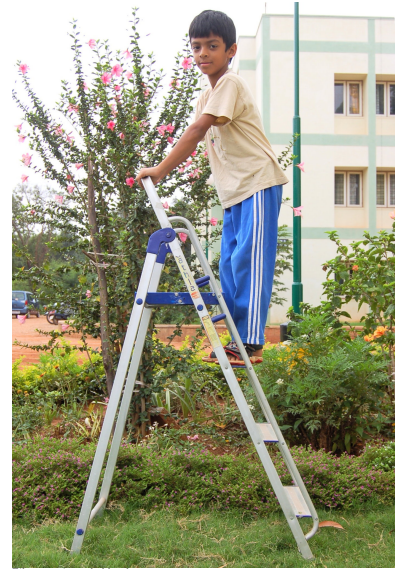
Figure 5.52: A ladder is well modeled as a collection of rigid pieces connected by pin joints ...
